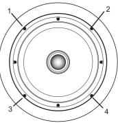
Tighten all four of the mounting screws in the same manner until the speaker is properly aligned and held tight to the wall surface. *Caution:* Do not over thighten!
